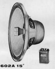
A companion piece to the 601A and identical in every way with the exception that it is mounted on a 15" frame and uses a 15" cone with a larger low frequency magnet for more efficient reproduction of very low frequency bass.
